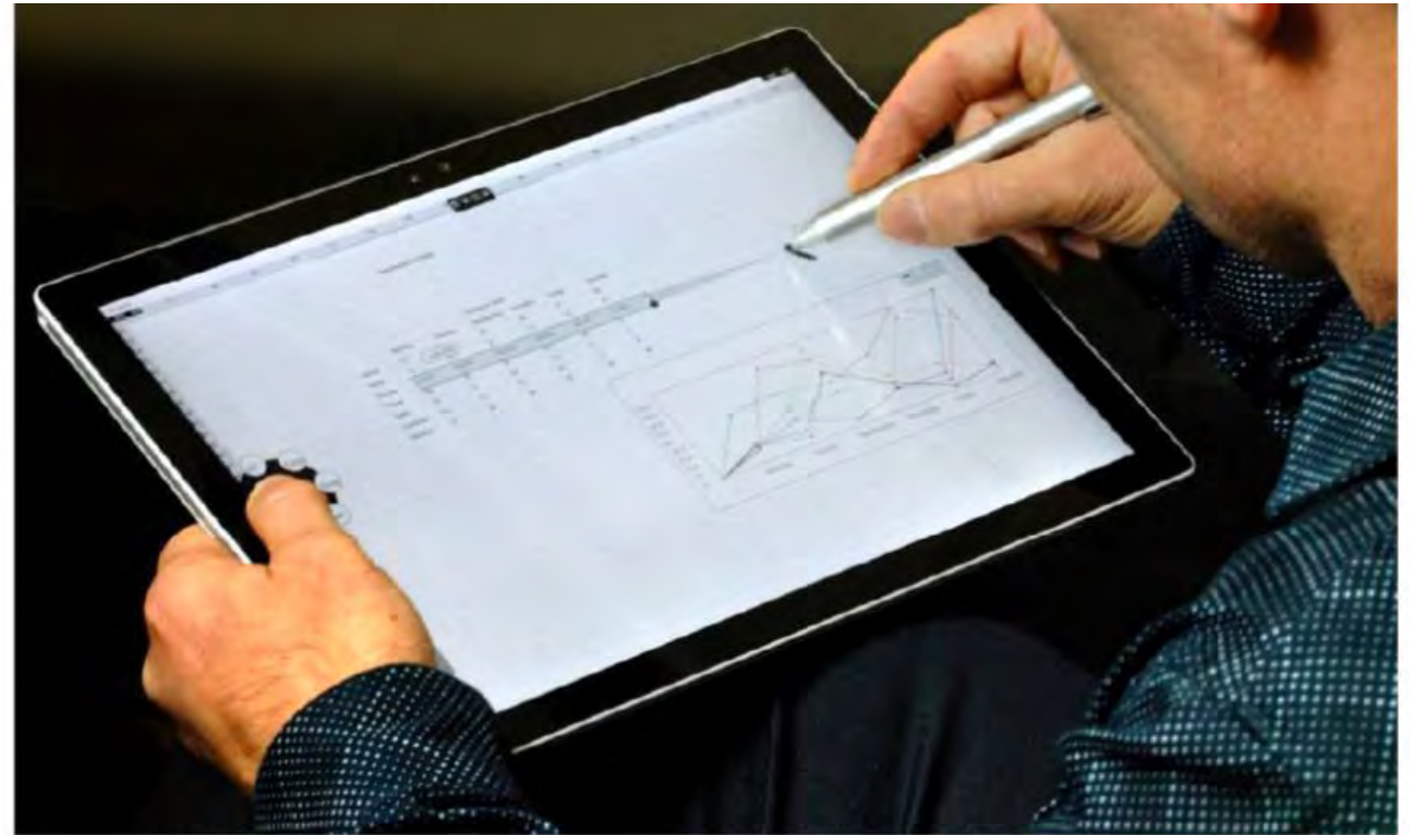
Figure 1: Thumb + Pen interaction enables simultaneous bimanual pen+touch while holding a tablet with the off-hand.
